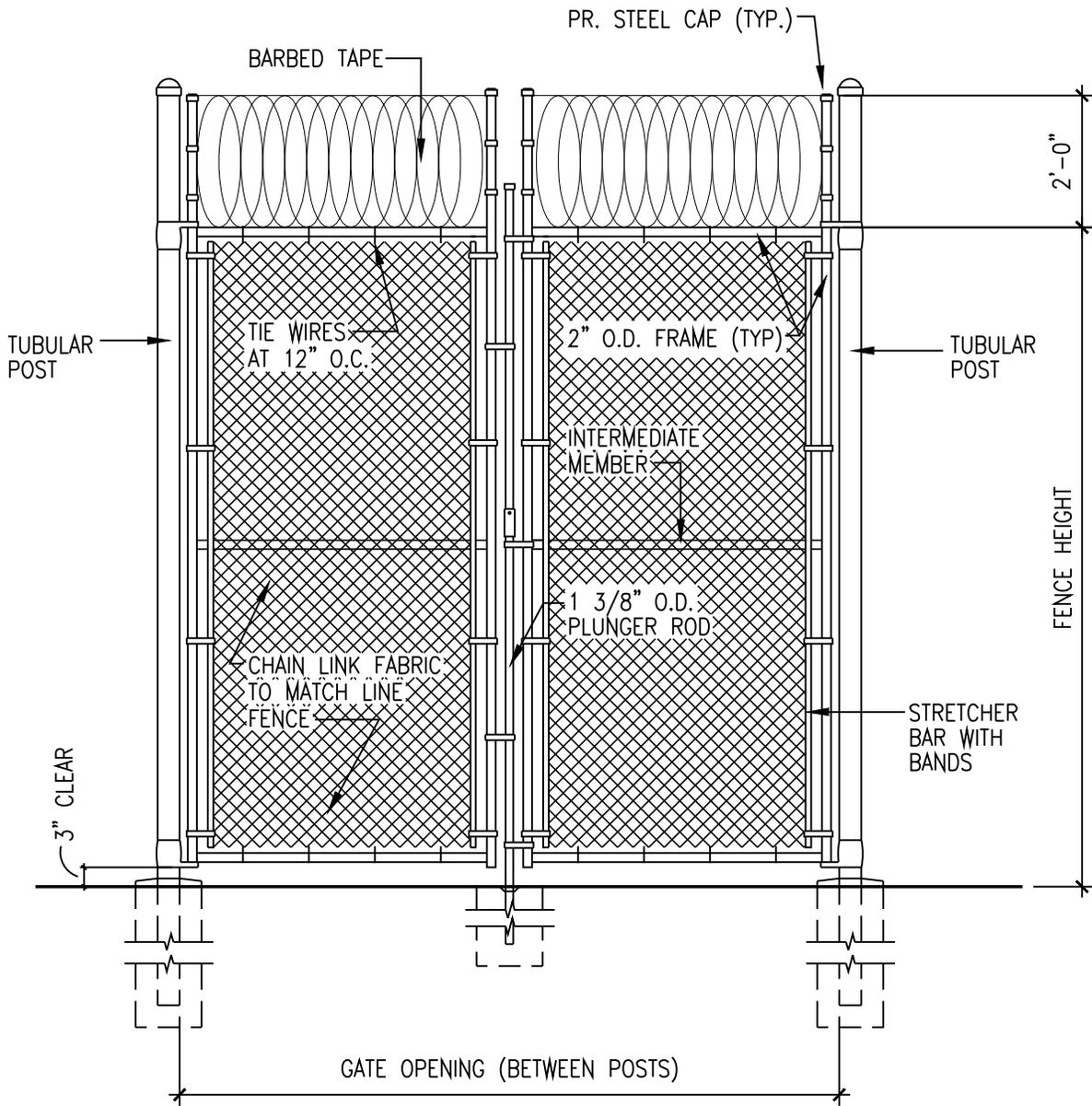
NOTE: GATE POSTS SHOWN ARE TO ILLUSTRATE HINGE ATTACHMENT. SEE WRITTEN SPECIFICATION FOR SIZE AND WEIGHT.
