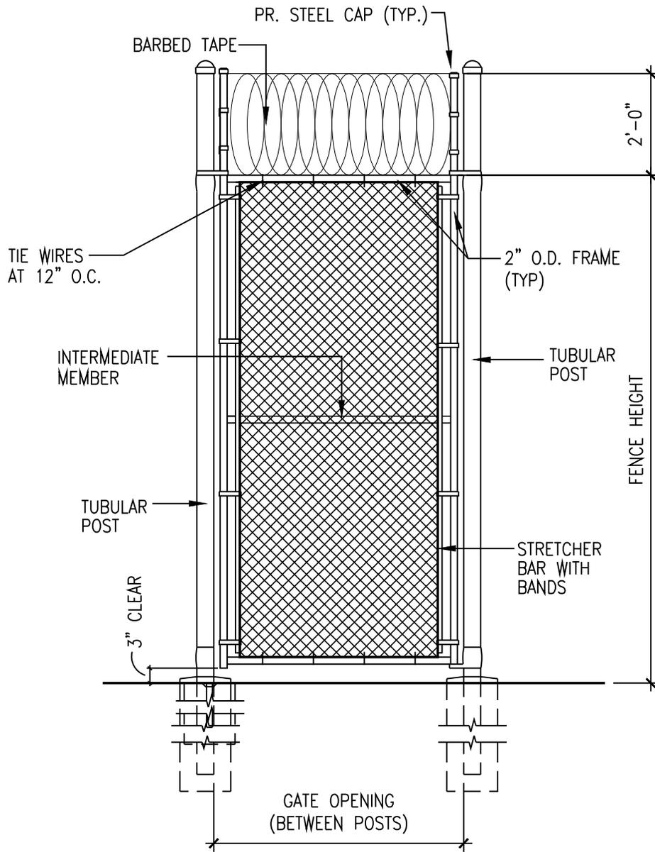
NOTE: GATE POSTS SHOWN ARE TO ILLUSTRATE HINGE ATTACHMENT. SEE WRITTEN SPECIFICATION FOR SIZE AND WEIGHT.
