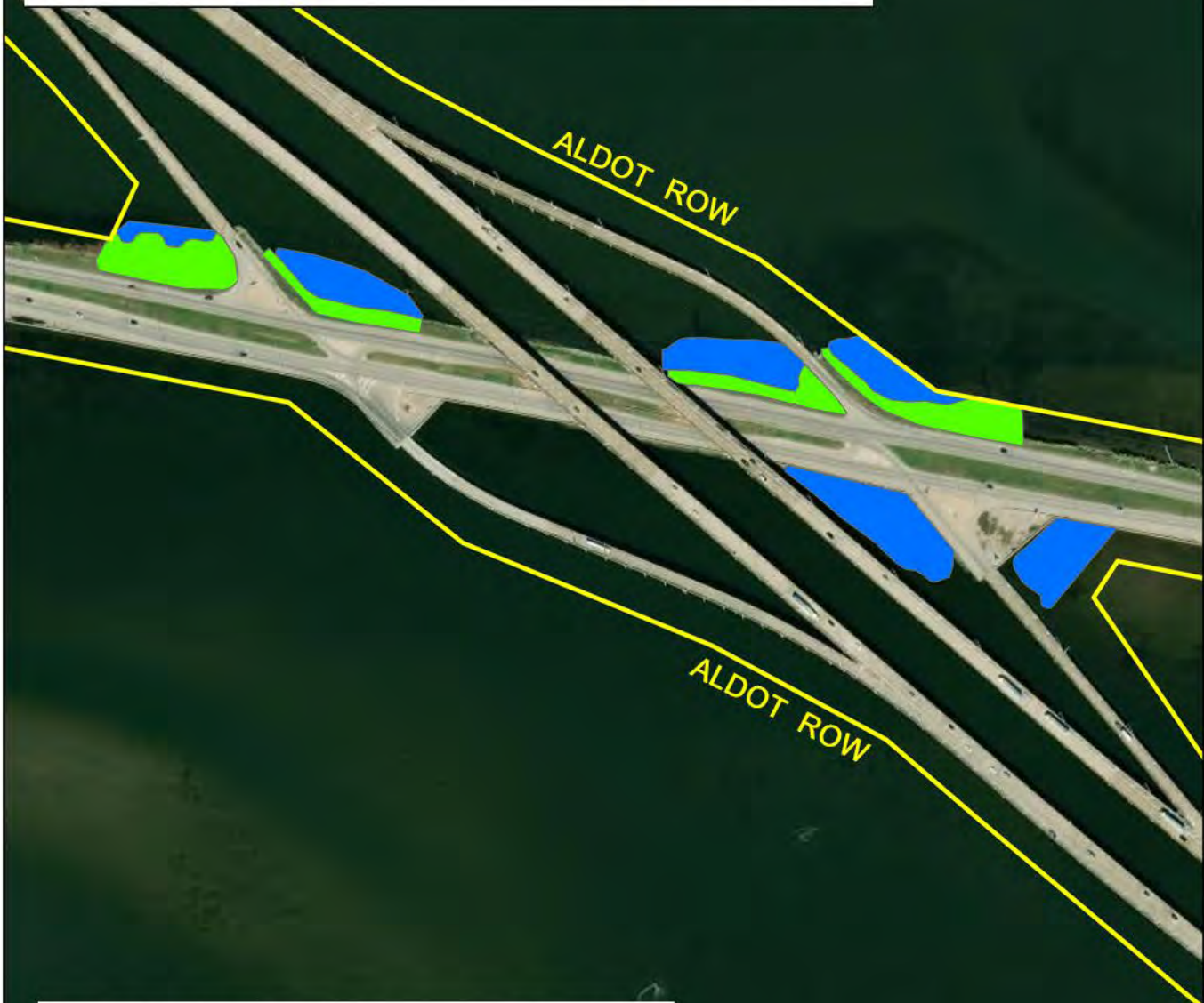
Figure 2B. Area of potential permanent impacts.
