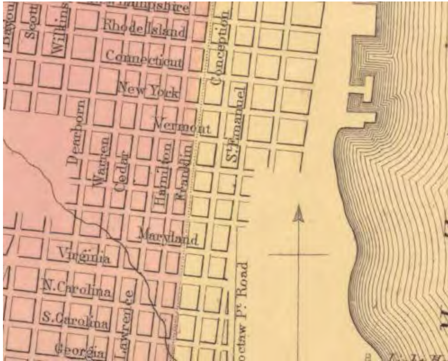
Figure 18. This 1867 map by Mitchell shows the dry dock at the foot of Connecticut Street also existing in 1853, as shown on a map drawn by Robertson of that year. An additional unknown wharf was newly constructed between 1853 and 1867, located at the foot of New York Street.
