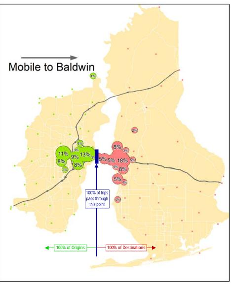
Figure 3-5 - Vehicles crossing Mobile Bay via US-98 per StreetLight Data
