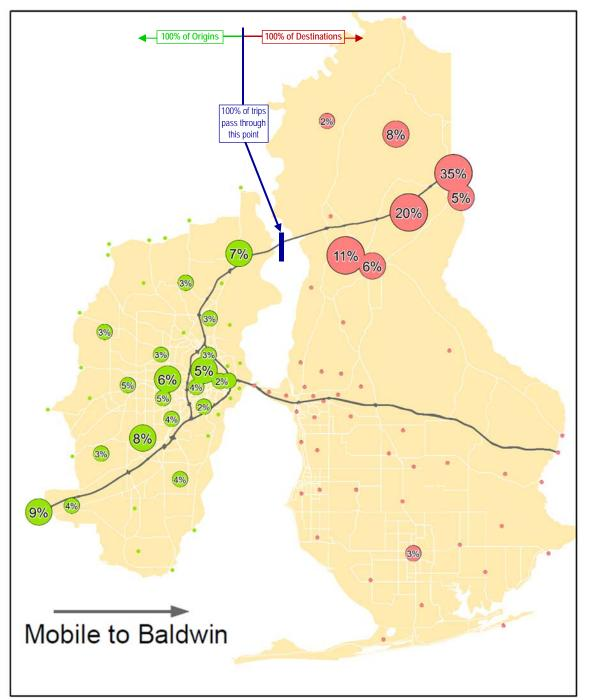
Figure 3-3 – Vehicles crossing Mobile Bay via I-65 per AirSage
