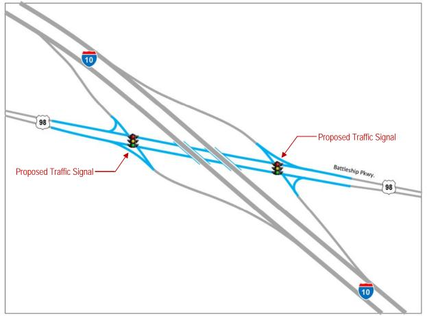
Figure 7-5 – Location D: Proposed Mid-Bay Interchange Configuration
